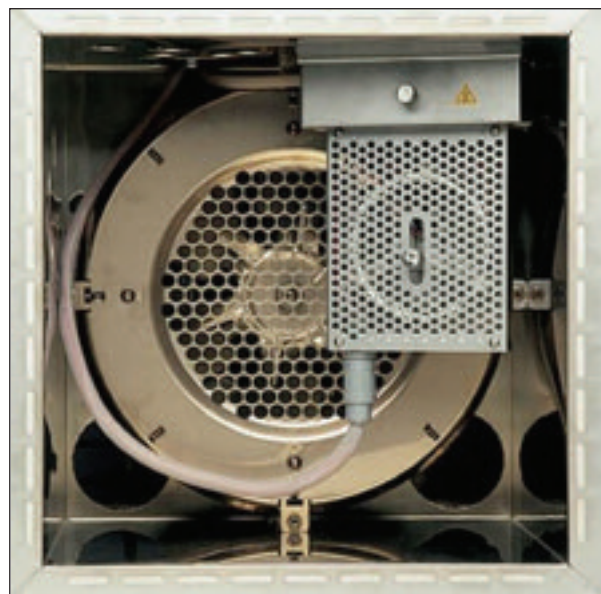
Figure 3: UFM column module housed in the TRACE GC Ultra oven.
