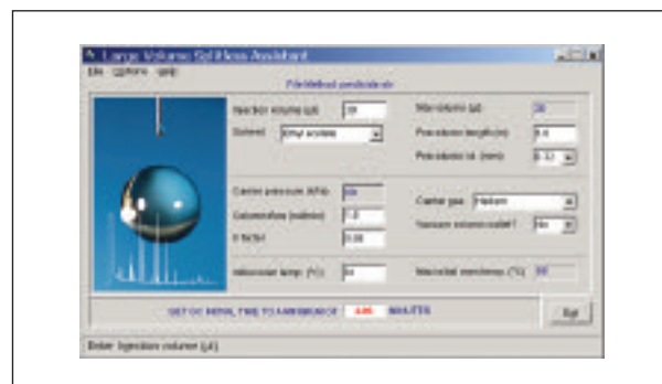
Figure 2: First screen of the LV-SL Assistant with determination of oven method parameters suitable for the injection of a 30 \mu\text{L} pesticides solution in ethyl acetate. This software provides the maximum initial oven temperature for a solvent at given conditions of carrier gas pressure and calculates the minimum initial oven time.
