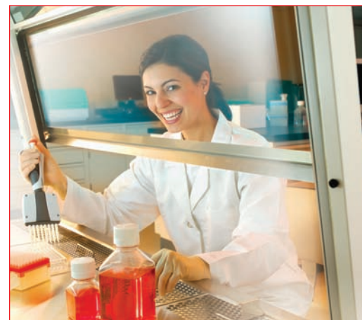
Figure 3. Transparent side walls introduce natural light into cabinets and reduce the sense of confinement associated with opaque side walls.
