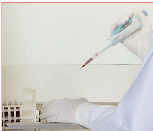
Figure 2. White back walls reduce glare.
