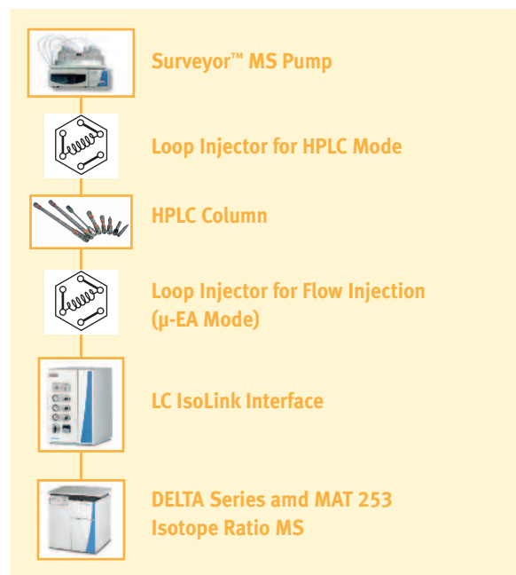
Figure 2: Scheme of the Thermo Scientific irm -LC/MS system with the LC IsoLink.
