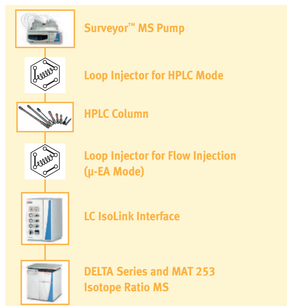
Figure 2: Scheme of the Thermo Scientific irm -LC/MS system with the LC IsoLink.
