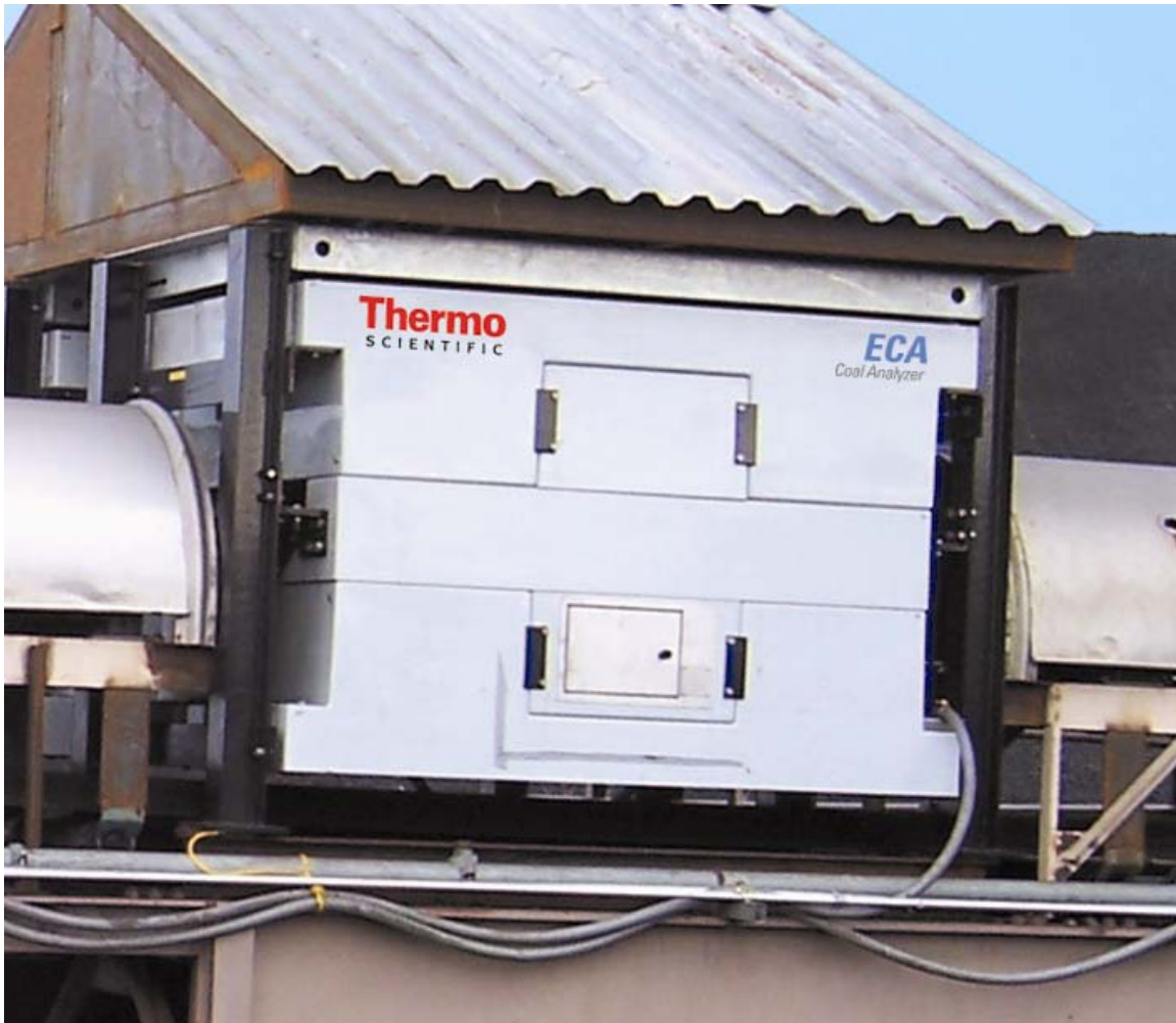
Figure 2: Thermo Scientific ECA, a full flow PGNAA analyzer, here seen in tandem on bunker feed conveyors
