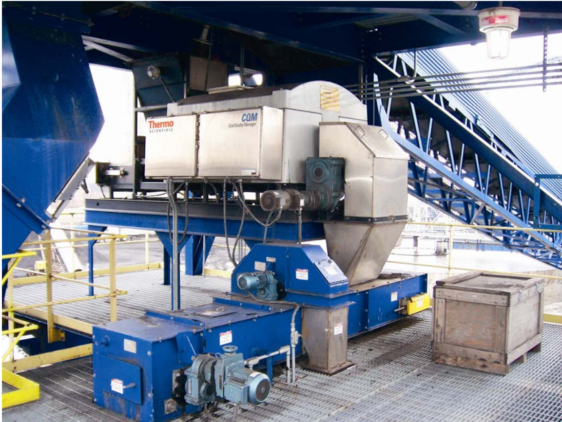
Figure 1 : Thermo Scientific CQM, a fixed geometry PGNAA coal analyzer designed for optimum precision
