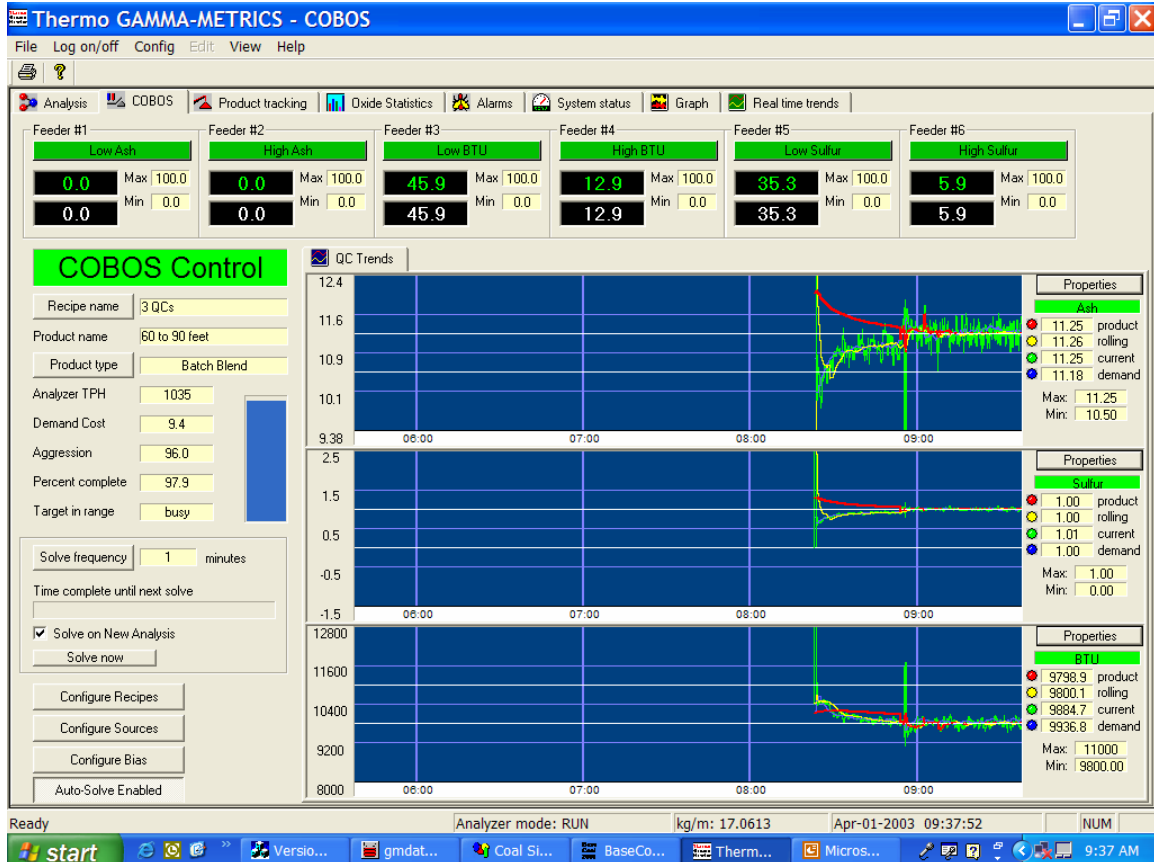
Figure 4: Thermo Scientific COBOS automated blending software, able to meet multiple control targets such as ash, sulfur and BTU/lb simultaneously
