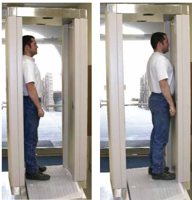
PM-7 Operation in Two-Side Measurement Mode: User measures back, then front, in two steps
