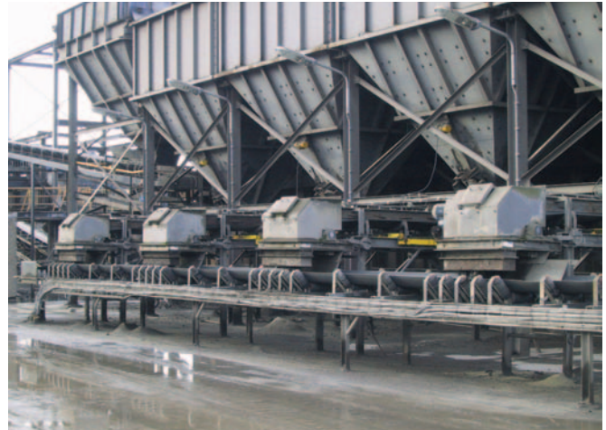
Figure 3: A weigh belt feeder along with a digital feeder controller provides accurate measurement and control of materials down to \pm 0.5\% .
