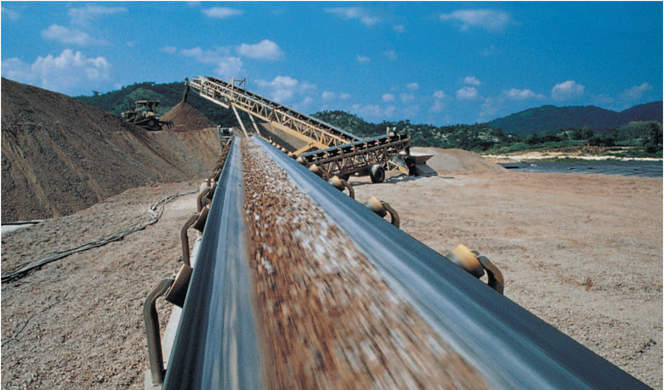
Figure 1: In-motion belt scale systems are used for providing accurate weighing measurements of materials from the moment they come off the truck and are crushed and screened, to the moment the final product is loaded back into the vehicle to leave the plant.
