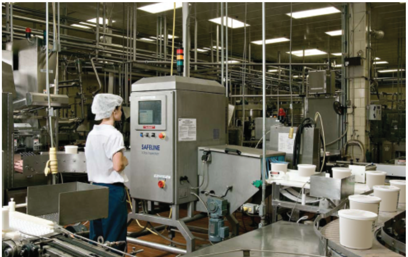
X-ray inspection easily detects contaminants during processing.
