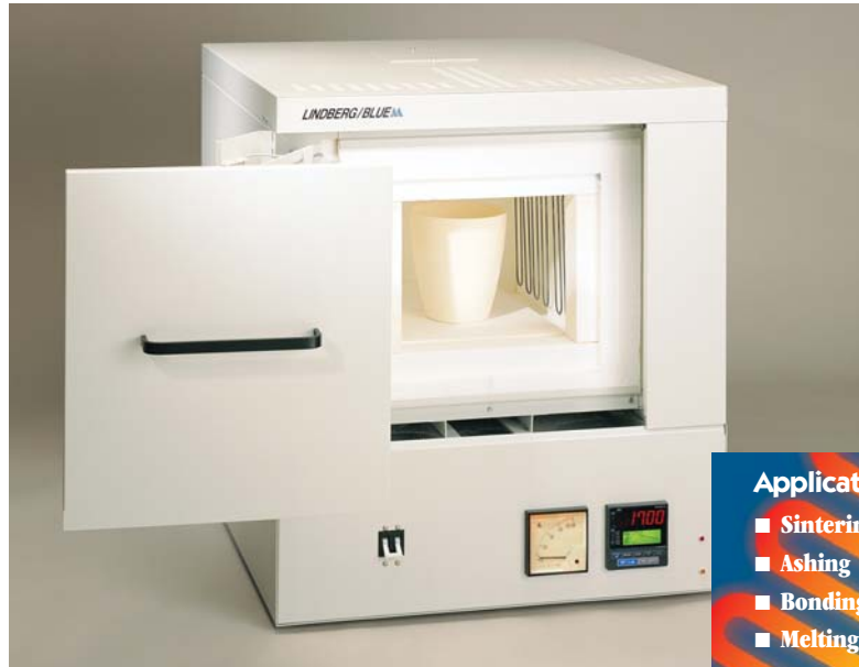
Integrated controls are standard on the large chamber, 1700°C Box Furnaces. Models available in 0.6 and 0.9 cu.ft. capacities. Model BF51634C shown.
