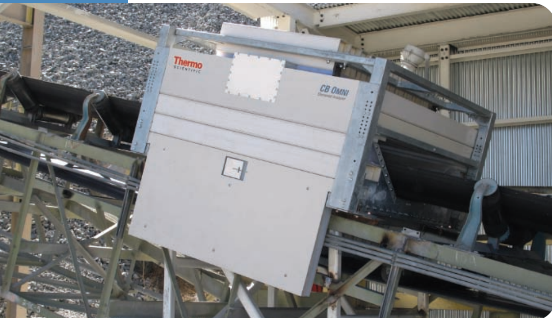
CB Omni CrossBelt online elemental analyzer
