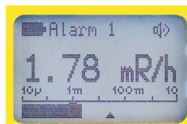
Alarm level 1 exceeded "Alarm 1" and "speaker" signs show up Absence of trend arrow indicates stable radiation level - reading can be taken
