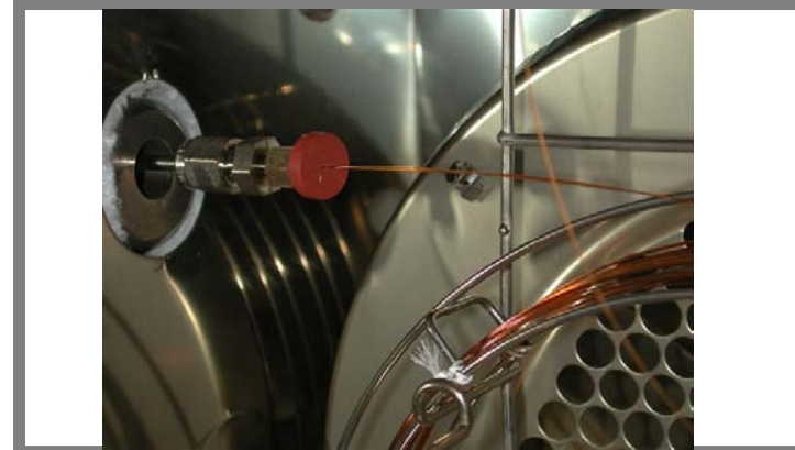
FIGURE 3. Close-up view of the LP-PCI acetonitrile fused silica line and GC capillary columns positioned through the GC transfer line
