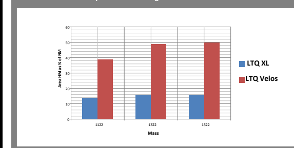
FIGURE 5. Comparison of the Relative Ejection Efficiency between the LTQ XL and LTQ Velos Ion Trap 4000 Mass Range.
