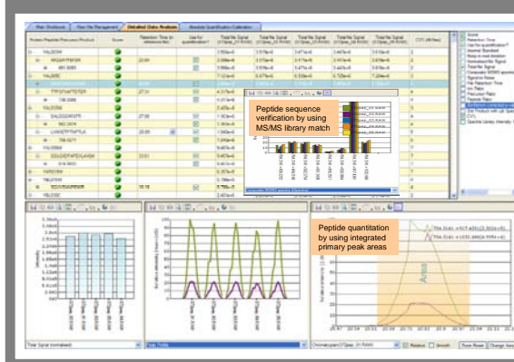
FIGURE 6. Peptide sequence verification and quantification using Pinpoint software
