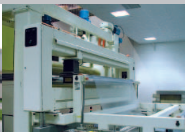
Thermo Scientific MARKIII Scanner on the Pharmaceutical Calender Line
