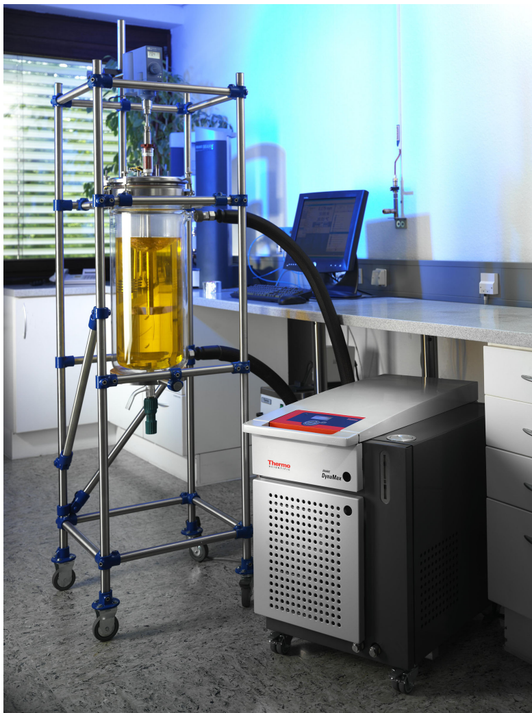
Figure 1: HAAKE DynaMax System and Reactor Vessel
