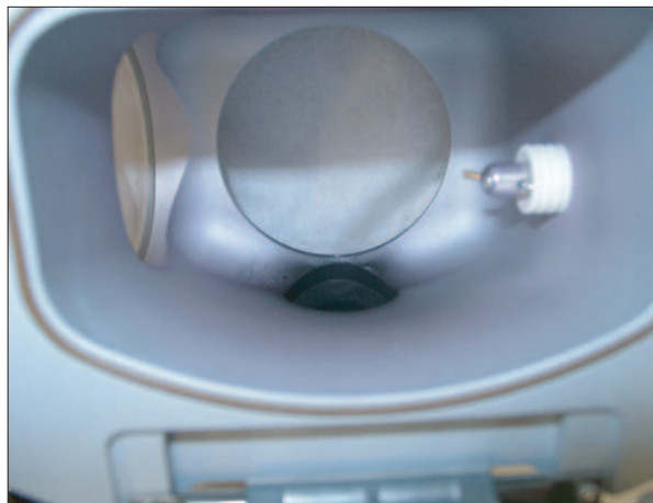
Figure 3: Electrospray ionization source with the electrospray probe removed, showing the main spray pattern directed towards the drain
