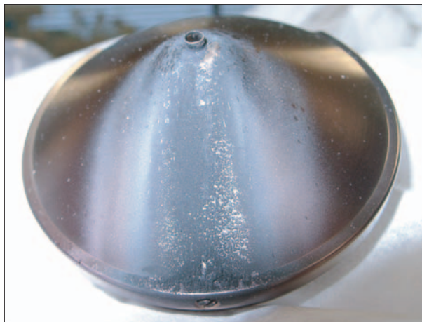
Figure 2: Ion sweep cap after several hundred injections, showing contamination from red wine
